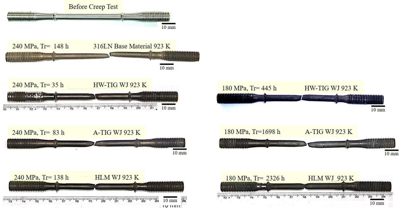
Fig. 15—Creep ruptured specimens tested at 923 K depicting the fracture location with reduction in ductility.
