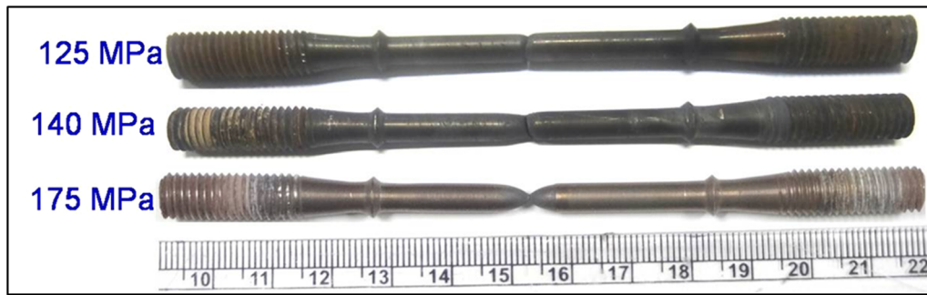
Fig. 10—Creep fracture location of the EB welded dissimilar weld joint specimens tested at 873 K.
