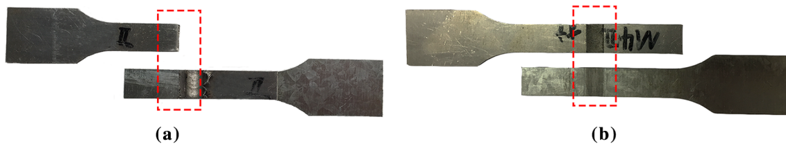
Fig. 7—Fracture position: (a) fracture position of P2, (b) fracture position of P1, P3, and P4.
