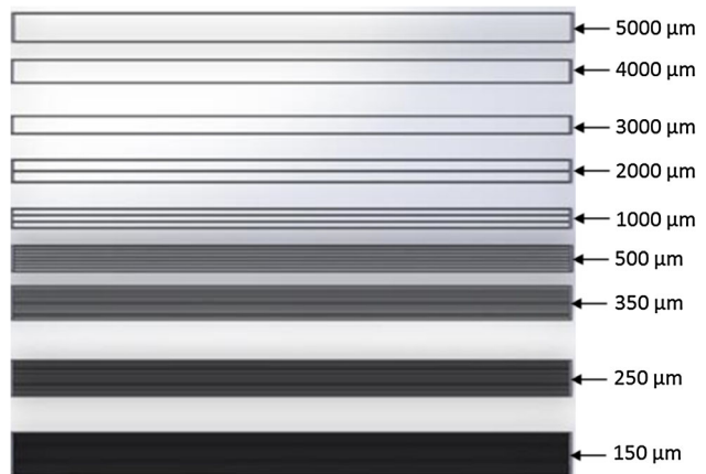
Fig. 2—Top-down view of heat-affected-zone experiment #2: 5, 4, 3, 2, 1 mm, 500-, 350-, 250-, and 150- \mu\text{m} -wide channels separated internally by 150- \mu\text{m} -thick walls.
