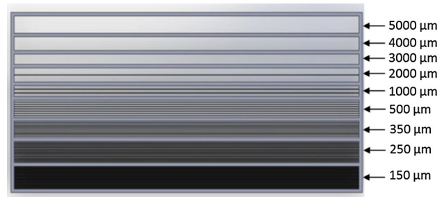
Fig. 1—Top-down view of heat-affected-zone experiment #1: 5-, 4-, 3-, 2-, 1-mm-wide, 500-, 350-, 250-, and 150- \mu\text{m} -wide channels separated internally by 100- \mu\text{m} -thick walls.
