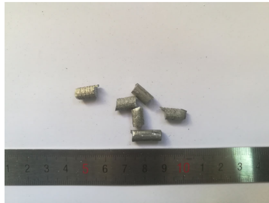
Fig. 2—Image of the Al/CNFs master alloy.
