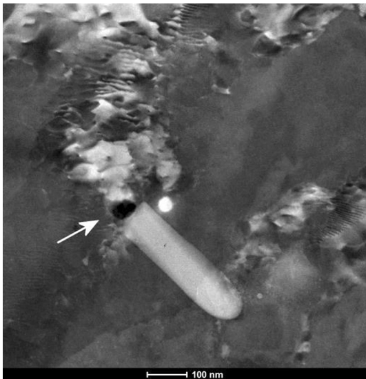
Fig. 6—TEM micrograph of Alloy-5 H18 with 0.99 pct Mn and 0.16 pct Fe showing a rod-shaped \text{Al}_6(\text{Mn,Fe}) dispersoid with a void generated in the end of long axis.
