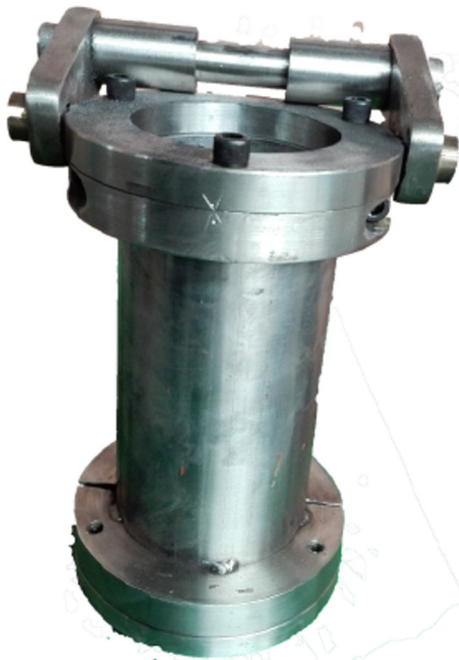
Fig. 3—Stainless steel cylinder with hanging system.
