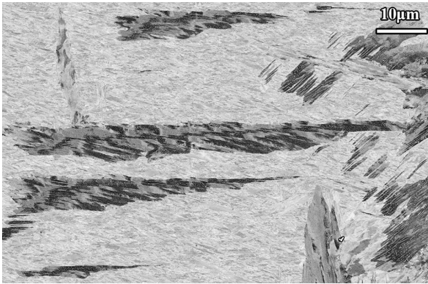
Fig. 7—Four parallel packets of ferrite plates from Fig. 5, which are now aligned horizontally. ECCI from an Fe-0.7C alloy held for 10 s at 773 K (500 °C).
