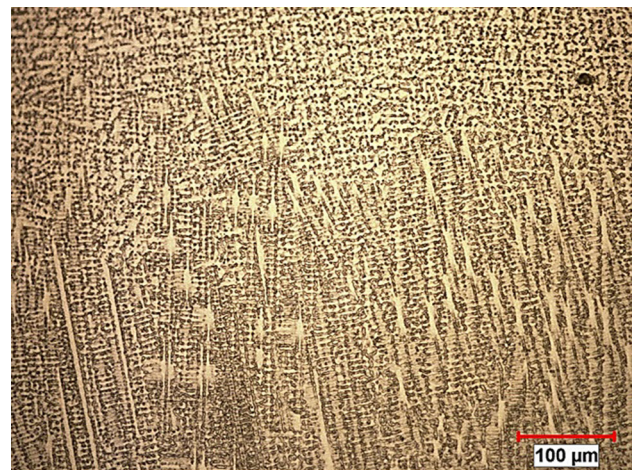
Fig. 6—Optical micrograph showing the solidification microstructure of a single-layer deposit.
