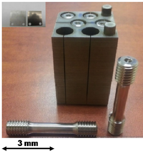
Fig. 1—H230 TLP-bonded stack and tensile testing specimens machined from the stack. The inset shows the H230 sheets before they are bonded.
