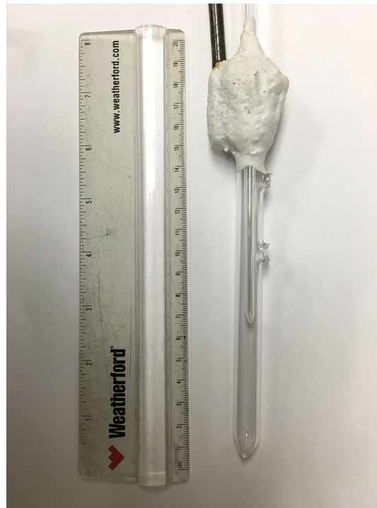
Fig. 1—A tubular quartz mold used for quenching experiment.
