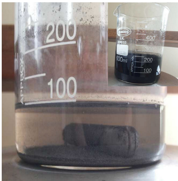
Fig. 12—Color change of Al–CNT suspension from dark to transparent at the end of mixing process.
