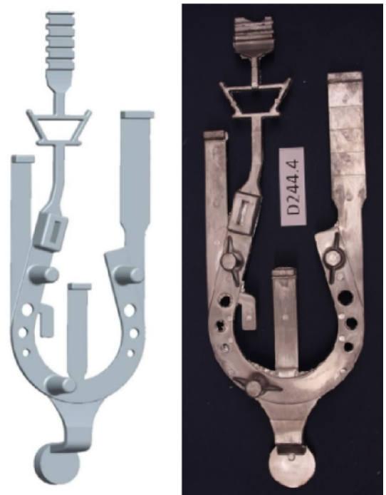
Fig. 2—Horseshoe-shaped casting designed to exacerbate the generation of defects as a function of the process parameters.
