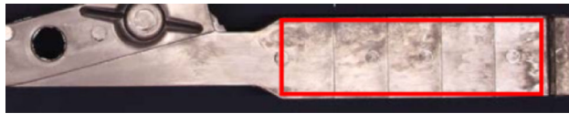
Fig. 4—Position of specimen for radiographic testing in the stepped wedge of the casting.
