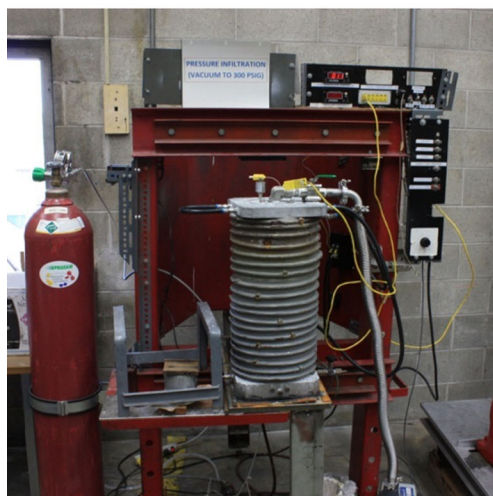
Fig. 4—Gas pressure infiltration equipment and its schematic.
