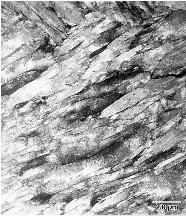
Fig. 7—TEM micrograph of the ferritic lath structure produced at a very slow cooling rate of \Delta t_{8/5} = 9983 s (0.016 °C/s).
