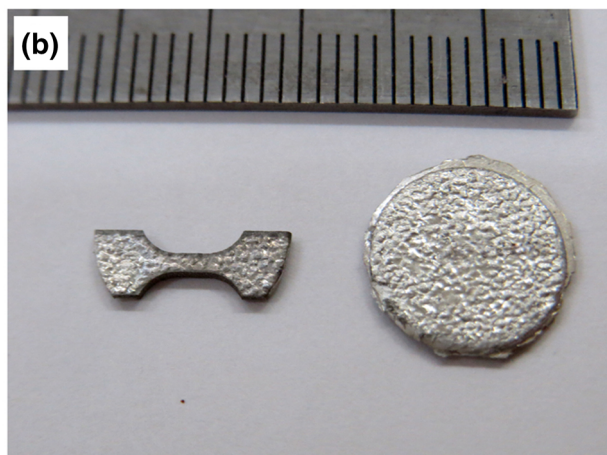
Fig. 2—(a) A schematic illustration of the HPT process and (b) A HPT disk with a tensile test sample.
