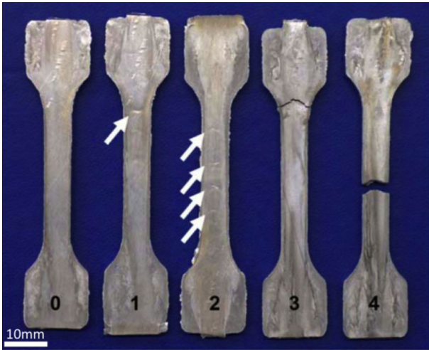
Fig. 2—Picture of a series of flat tensile test pieces each of which is representative of one of the categories in the hot-tearing scale defined (the reference number corresponding to the scale is indicated at the bottom of each). The white arrows indicate the surface dimples that are associated with internal cracking (see also Fig. 3).
