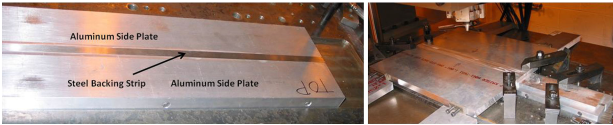
Fig. 10—Picture of composite backing plate (left). Weld setup with composite backing plate (right).
