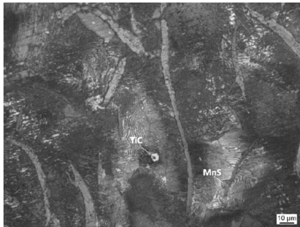
Fig. 5—Color-etched micrographs of the sample. 621.1—0.018 pct S, 0.06 pct Ti at high magnification.
