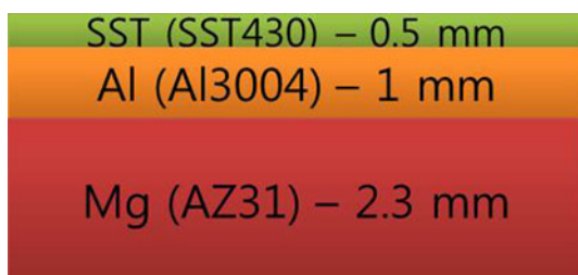
Fig. 1—Configuration and dimensions of AZ31Mg/3004 Al/SST 430 plates.
