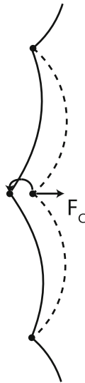
Fig. 5—Schematic representation of an atom jumping against the cusping bias F_C b .
