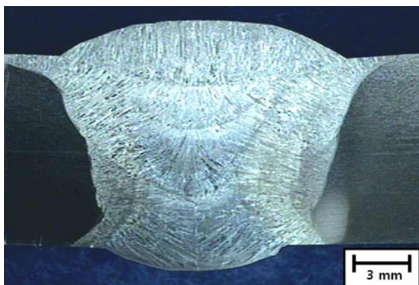
Fig. 5—Macrograph of the four-pass weld joint.
