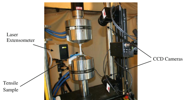
Fig. 1—A 3-D digital image correlation system integrated on a MTS testing frame. CCD , charge-coupled device.
