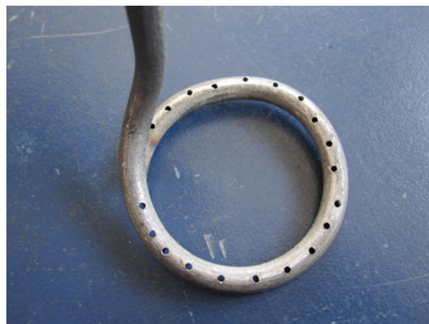
Fig. 10—Apparatus for stirring in LiCl-KCl-AlCl 3 (0.247 mol L -1 ) on a solid Fe electrode at 723 K (450 °C) with flow rate of 0.3 L min -1 .
