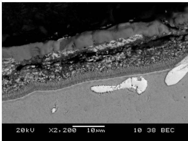
Fig. 14—SEM micrograph of a Gleeble-simulated material rapidly heated to 1548 K (1275 °C) and held for 2.5 s.
