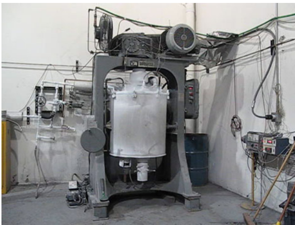
Fig. 1—Cryomilling of 20-kg batch at DWA Aluminum Composites (Chatsworth, CA) using modified Szegvari attritor (courtesy of Mark van den Bergh).
