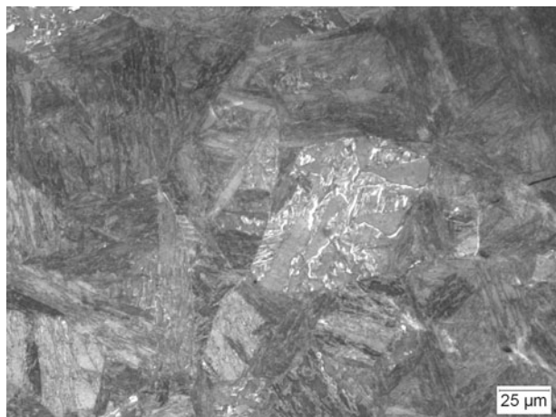
Fig. 10—Presence of retained austenite in the BA-160 CGHAZ sample revealed as white films along martensite lath boundaries.
