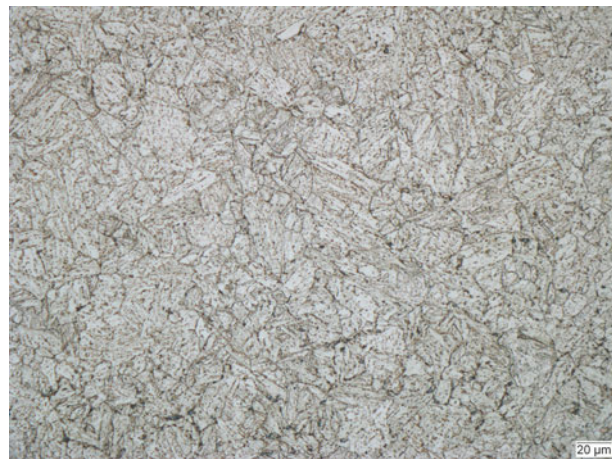
Fig. 1—Microstructure of BA-160 BM in the heat-treated condition with measured hardness of 402 HV.
