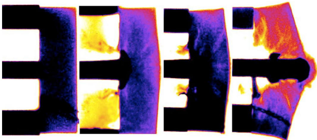
Fig. 3—X-ray image showing a steel rod 10 mm in diameter hitting a block of glass at a velocity of about 500 \text{ m s}^{-1} . The first image was taken 3 \mu\text{s} after impact, and the second 30 \mu\text{s} later. By the third frame, the rod has eroded a pit in the glass and the block begins to fail. In the final frame, 80 \mu\text{s} after impact, a disc of metal sheared off by the glass can be seen left behind in the surface crater.
