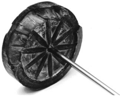
Fig. 6—Butt and fragment of extruded aluminum wire. Wire diameter 1.5 mm ( \lambda = 711 , T = 293 K (20 °C)).
