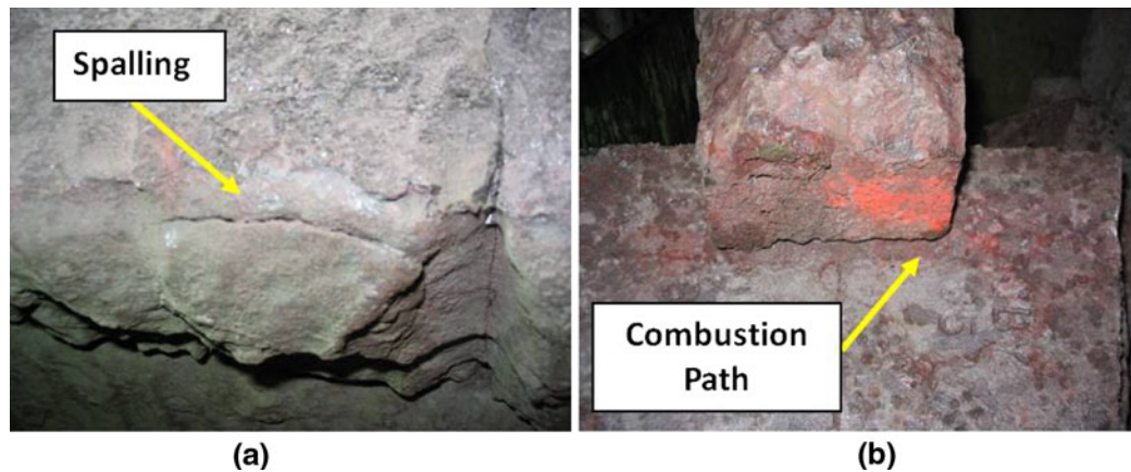
Fig. 12—Dome hot-face refractories. (a) Side view showing spalling where bricks join and showing surface spalling in the process of occurring, and (b) path of carbon feedstock that has entered between joints of the refractory, “combusting” between brick layers. Note the different shades of color at the brick joints where slag is present, which is caused by slag iron in different oxidation states in (b). A combustion pathway is evident at the side and base of the bricks. In (b), the single brick on top is from the hot face and the two bricks underneath are from the backup lining.
