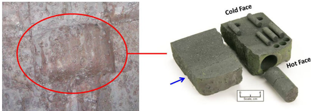
Fig. 16—Cross section of a 90 pct chrome oxide refractory removed from a gasifier sidewall using coal as a feedstock after approximately 4000 h of usage between 1673 K and 1773 K (1400 °C and 1500 °C). Note the slag penetrated area on the hot face, along with the cracking occurring at the slag penetrated/not penetrated interface, indicated by the arrow.
