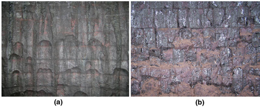
Fig. 13—Sidewall wear occurring on sidewall refractories containing approximately 90 pct chrome oxide. Figures (a) and (b) come from different gasifiers run under different operational conditions and indicate two different types of surface wear: (a) spalling occurring in large sections not limited to brick boundaries and (b) spalling of individual brick. Corrosion from slag occurs at the surface of both bricks.
