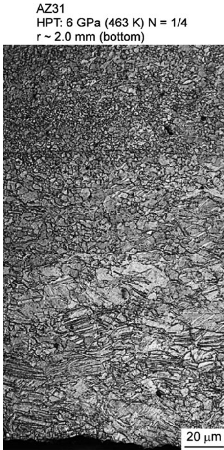
Fig. 5—Grain size heterogeneity on the cross-sectional plane of an HPT sample after 1/4 turn at 463 K (190 °C).
