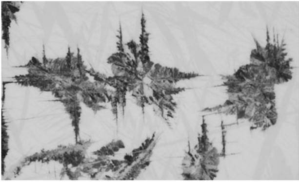
Fig. 26—Spiky nodules formed after 2 h at 548 K (275 °C) in steel with 1.67 mass pct C. Light micrograph at 900 times magnification.
