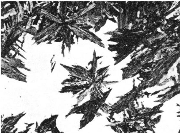
Fig. 13—Spiky nodules of inverse bainite formed after 60 s at 723 K (450 °C) in steel with 1.65 mass pct C. Light micrograph at 600 times magnification. From Modin and Modin.<sup>[17]</sup>
