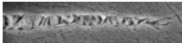
Fig. 35—Last leg of a zigzag pattern formed after 96 h at 473 K (200 °C) in a steel with 1.67 mass pct C. SEM at 30,000 times magnification.
