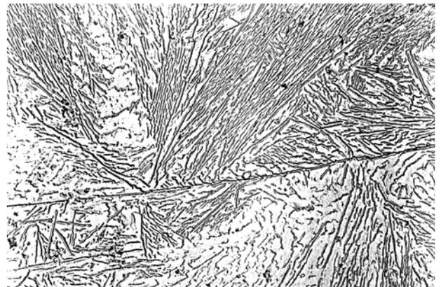
Fig. 18—Beginning of fan-like growth by branching of cementite plates. Formed after 600 s at 623 K (350 °C) in steel with 1.65 mass pct C. 4000 times magnification. From Modin and Modin.<sup>[17]</sup>
