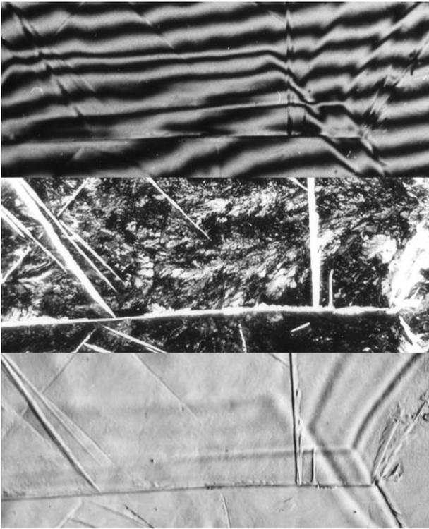
Fig. 2—Metallographic evidence of surface relief caused by Widmanstätten cementite formed during 300 s at 923 K (650 °C). Upper: interferogram; Middle: etched; Lower: unetched, oblique illumination. 400 times magnification. From Speich.<sup>[13]</sup>
