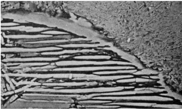
Fig. 12—Inverse bainite as counterpart of feathery bainite in Fe-1.7 mass pct C after 3 s at 723 K (450 °C). Electron micrograph of plastic replica at 12,000 times magnification. From Hillert.<sup>[1]</sup>
