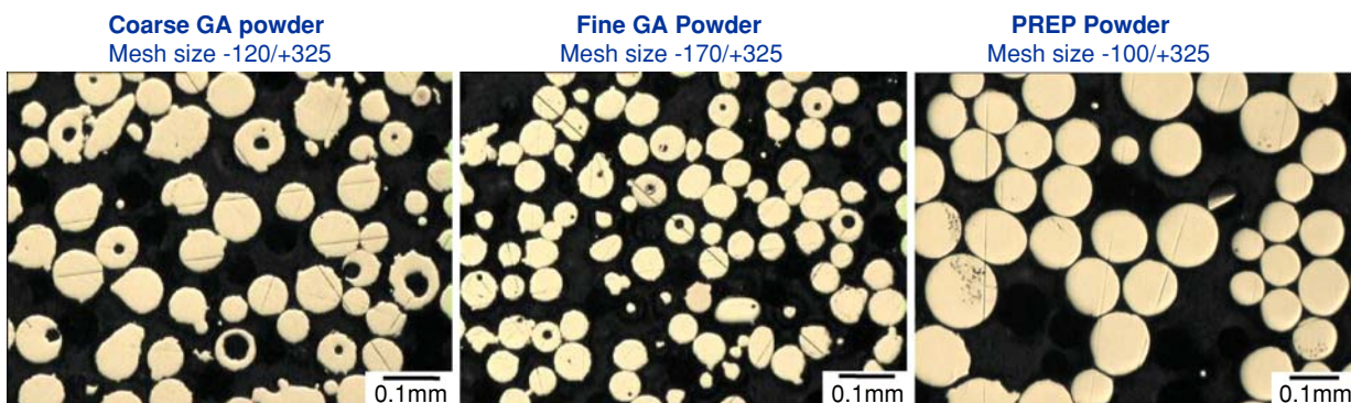
Fig. 2—Micrographs of the three types of IN718 powder used in this study.
