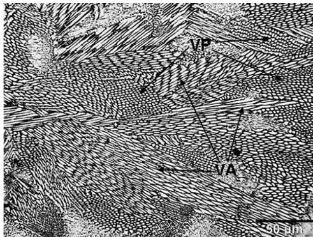
Fig. 4—Upper surface optical micrograph showing austenite solidification cellular microstructure including positions VP and VA to the axis of the columnar.
