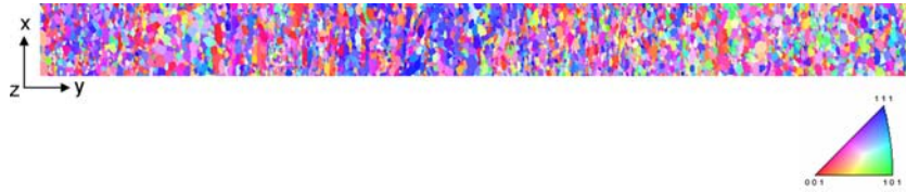
Fig. 6—Montage of EBSD crystal direction maps across thickness direction ( y ) of tantalum plate. Map color denoting crystal direction is with respect to y .
