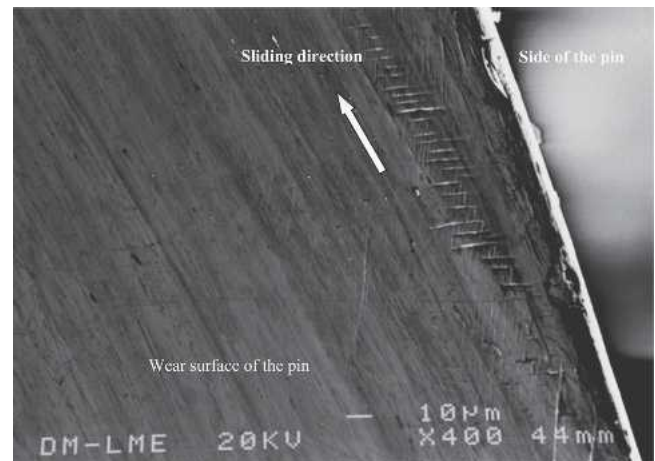
Fig. 9—Wear surface for alloy 21 at 20 N load and 0.2 m/s sliding speed, in which severe wear is not observed.
