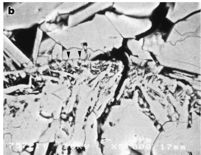
Fig. 12—Polished cross-sectional SE micrographs of the Fe-7.5 wt pct Al sample showing (a) the lenticular nature of the nodule and (b) the remnants of an original surface scale between the outer iron sulfide scale and inner mixed sulfide layer as indicated by arrows.
