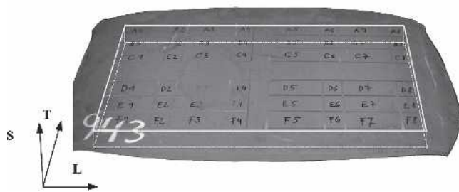
Fig. 1—Indexing of directions on the rolled plate according to ASTM E 399 [17] (here, low S material). Sections of microsamples are named after the direction of the normal of the section (compare with Figure 2).
