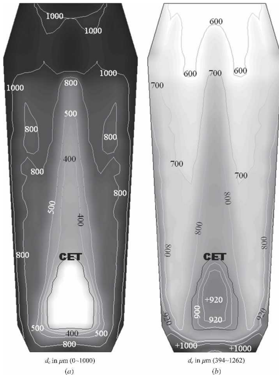
Fig. 5—Predicted columnar trunk diameters, d_c , and diameters of the equiaxed grains, d_e , for the 2-D axis symmetrical benchmark ingot. The quantities are shown with gray scales from minimum (bright) to maximum (dark), together with isolines. The CET is shown by the black line.
