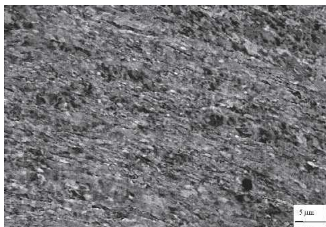
Fig. 10—Microstructure of material I after three passes of ECAE, as recorded using the scanning electron microscope (SEM) operated in backscattered detection mode.
