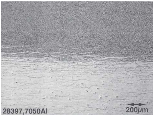
Fig. 8—Micrograph of friction-stir-processed 7050-T7451. The transition from the fine-grained microstructure produced by stirring into the unprocessed zone is clearly evident.
