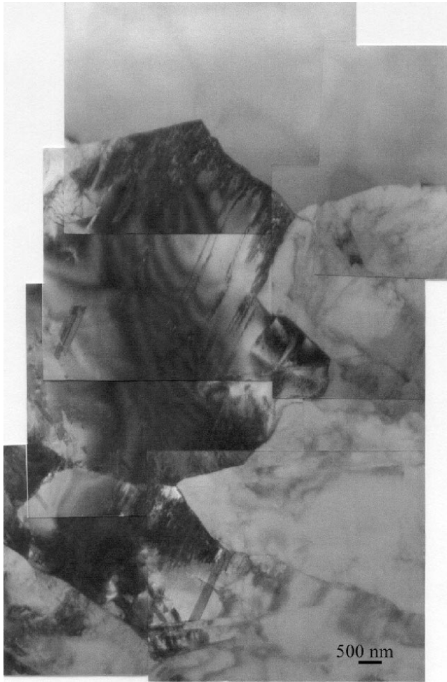
Fig. 14—A collage of TEM bright-field images revealing the overall microstructure of the water-quenched sample of alloy I.
