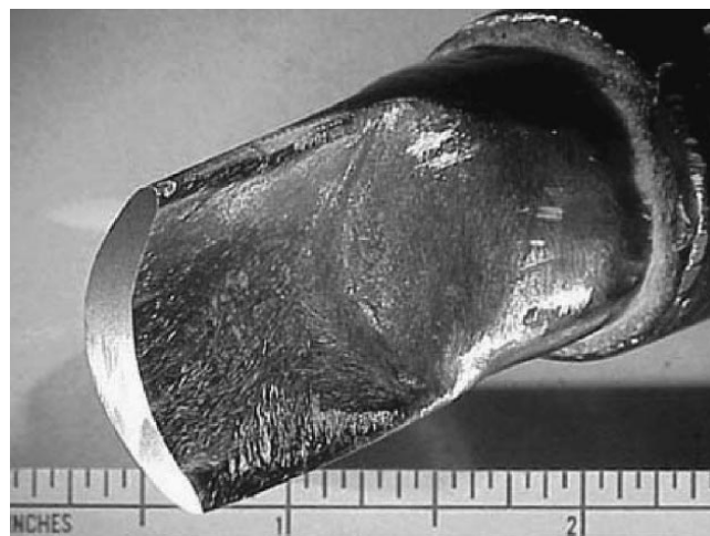
Fig. 3—Typical investment-cast Nb-silicide composite prototype airfoil based on a composition of Nb-22Ti-2Hf-4Cr-3Al-16Si, with minor additions of Ge and Sn.
