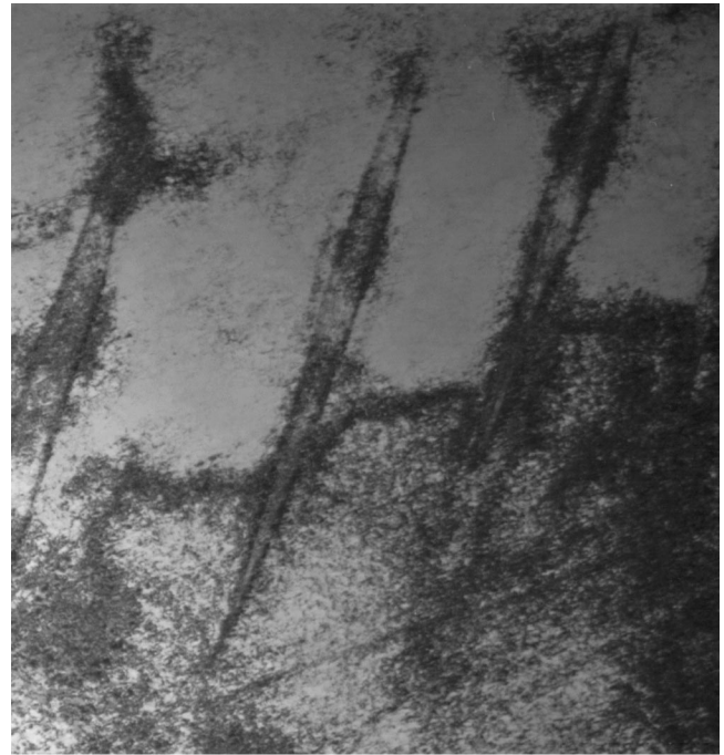
Fig. 3—TEM micrograph of NiTi overaged (823 K, 1.5 h) specimen [123] showing the precipitates and dislocations (after thermal cycling).
