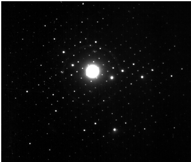
Fig. 5—TEM photomicrographs of hiped compact heat treated at 1150 °C for 3 h and water quenched showing (a) absence of dissolution of oxide particles, (b) an oxide particle (A) projecting from the matrix, (c) diffraction pattern taken from region (A), and (d) computer simulated key for orthorhombic structure with zone axis \langle 001 \rangle .
