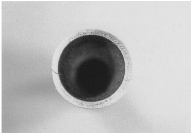
Fig. 4—Split that occurred during a flare test. Bottom view.
