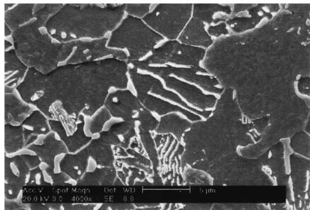
Fig. 11—Microstructure of AISI 1541 from the intercritical cycle after 4 h at 688 °C and cooling to room temperature. Note the 5 μm marker. The coarse pearlite was formed at 688 °C and the fine pearlite was formed during the final cooling rather than at 688 °C.
