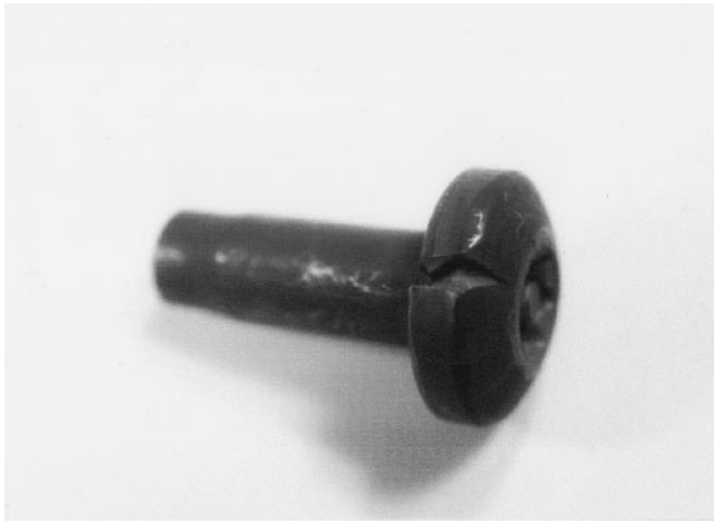
Fig. 1—Split that occurred during cold heading of a bolt.
