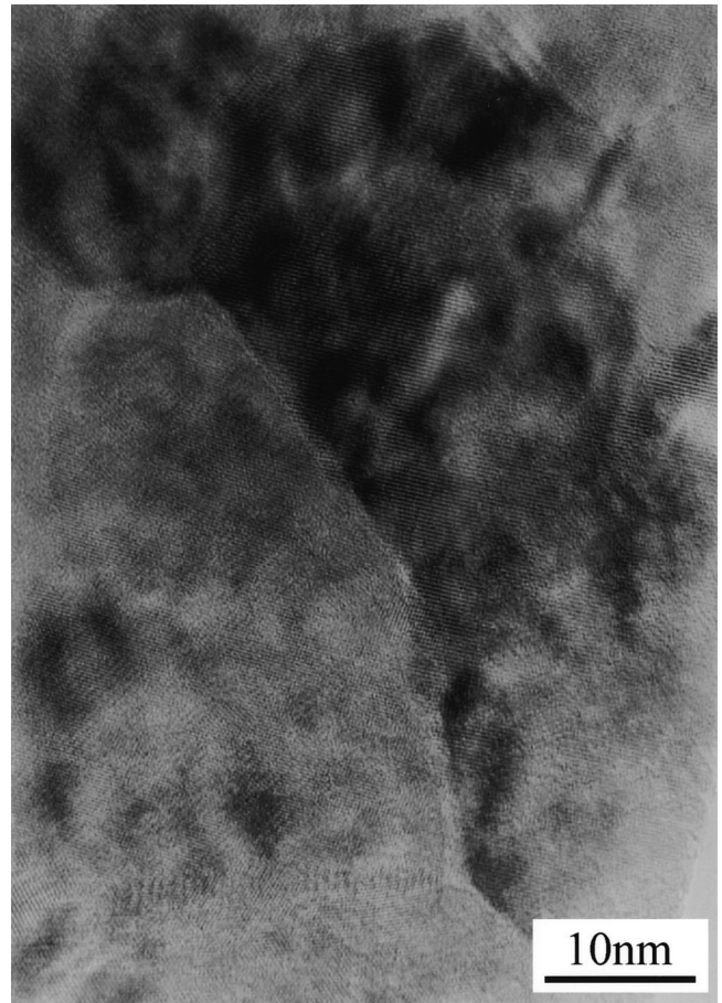
Fig. 9—HREM image of the nanocrystalline ferrite in the 360 ks ball-milled powders after annealing at 673 K for 3.6 ks.
