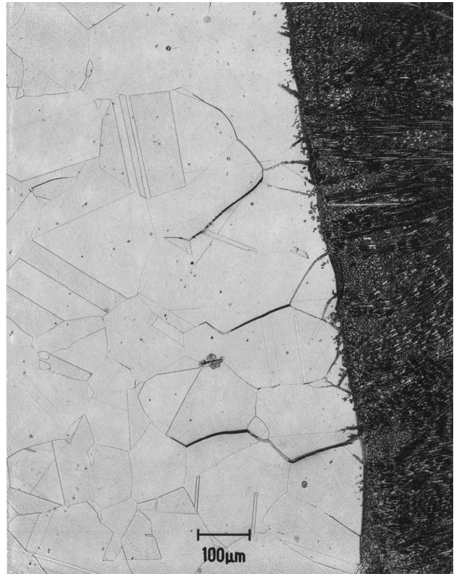
Fig. 11—SEM image showing microfissures in HAZ of high boron alloy subjected to the solution treatment at 1150 °C for 5.5 min and followed by air cooling.
