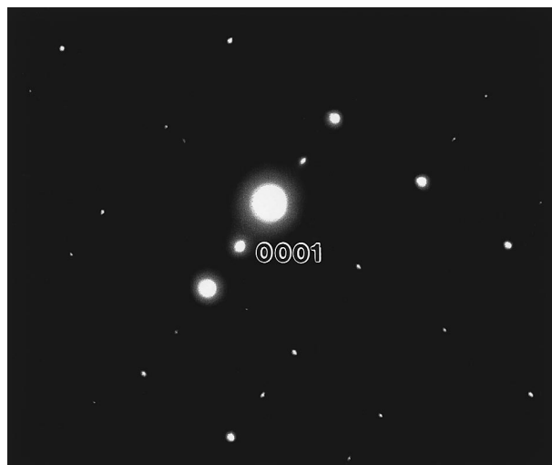
Fig. 1—Selected area diffraction pattern from [14\bar{5}0] zone axis of Q phase grain, showing the presence of (0001) reflections.
