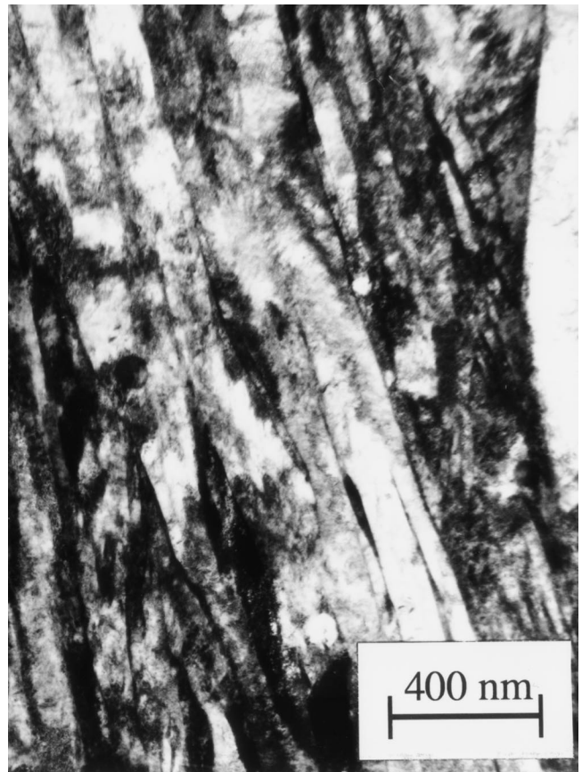
Fig. 10—TEM micrograph showing the characteristic lath of martensite.
